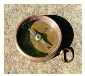
The compass is simple to use, just set it on a level spot and gently rotate until the swinging arrow lines up with North. Please be aware the computers and cell phones will affect the compass's ability to read true north.
