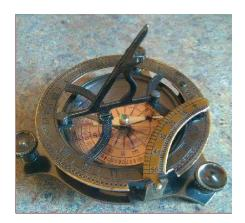
The small slide on the side freezes the needle to protect it during shipping. It needs to be freed to be able to use the compass.
